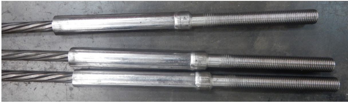
Figure 2. Swaged stud to attach the thread to the cable
