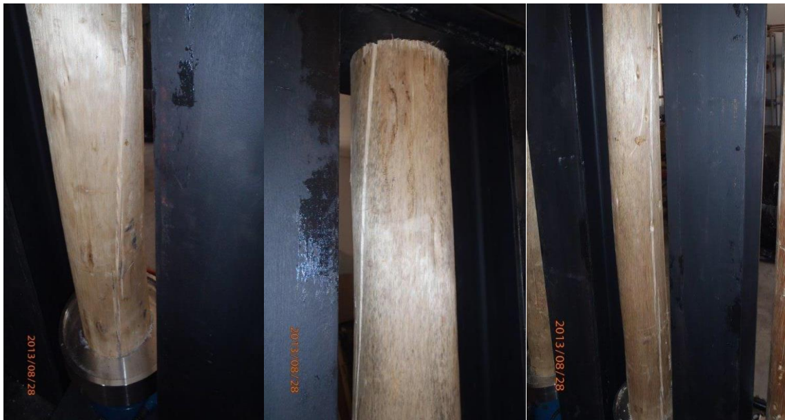
Figure 7. Photographs of Mine Poles in SLF with significant crack propagation
