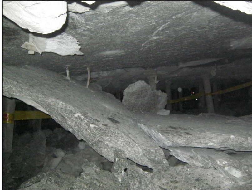
Figure 3: 8mW28W2 Note the smooth, flat fracture plane
