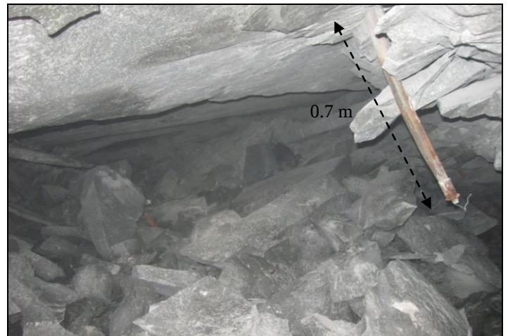
Figure 4: A 180t FOG in the face of a panel.
