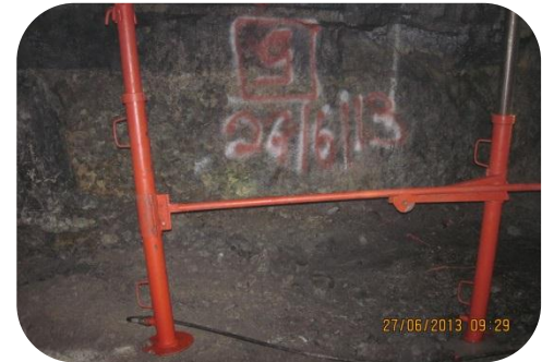
Guide rod and Hydraulic rod is secured to the unit requiring remote installation and moved forward along the guide unit to the desired position
