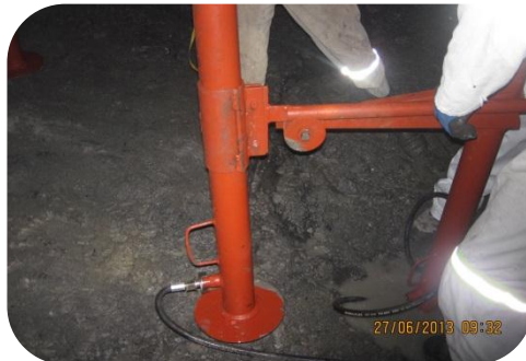
Depicting guide bracket, extension rod and bracket and hydraulic hose connection
