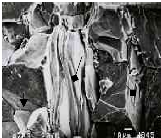
Figure 10: SEM micrograph illustrating general initiation and propagation of Inter-granular ( ➡ ) and Intra-granular ( ◆ ) cracks in Anorthosite samples stressed to 0.2UCS uniaxially
