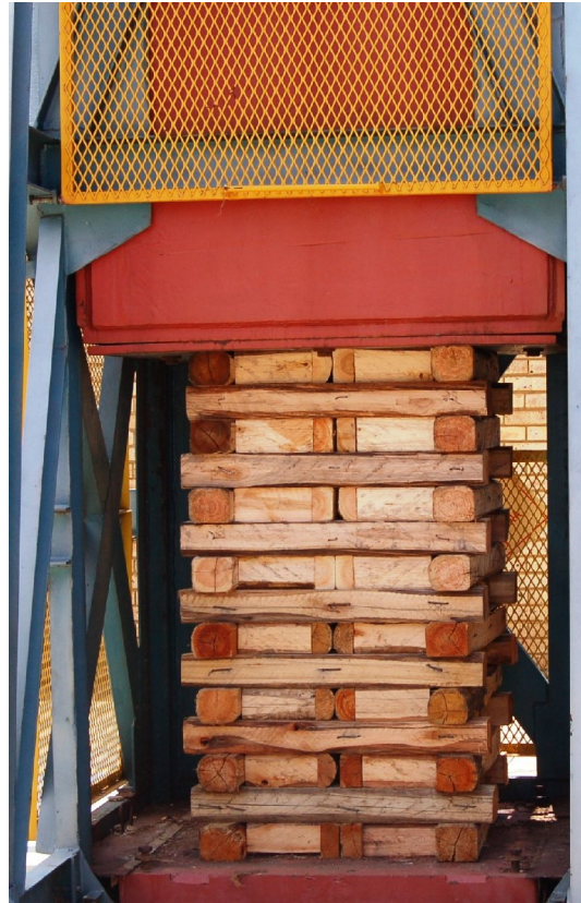
An Extended Lexus pack in the drop test facility of Reatile Timrite. The mass is 16 tons.
