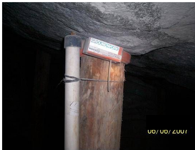
Figure 6. Load and Closure Logger installed on a mine pole
