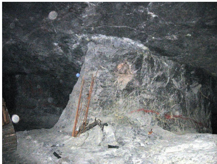
Figure 13. 3.5m high 4m x 6m pillar
