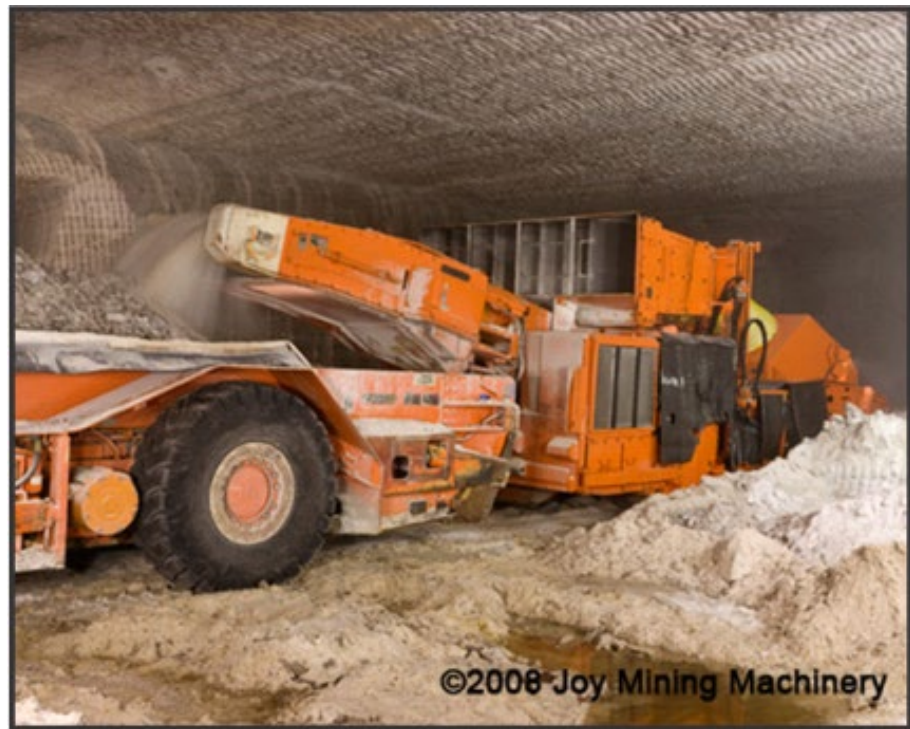
Figure 8: Shuttle car being loaded by a continuous miner (JOY Mining Machinery)
