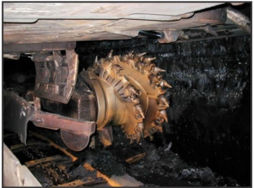
Figure 46: Mechanical coal cutter (Shearer)
