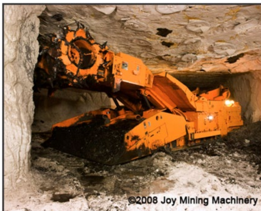
Figure 4:A continuous miner in a coal face (JOY Mining Machinery)
