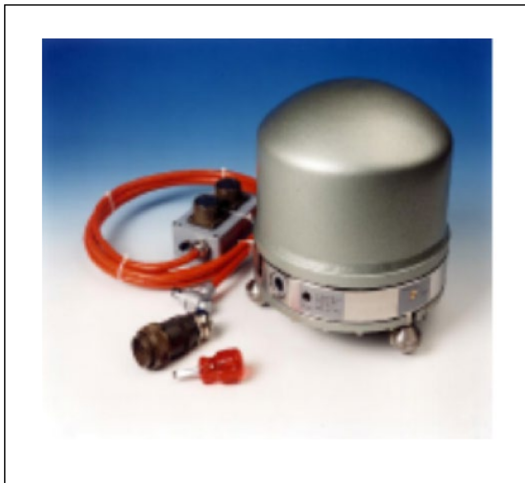
Figure 3: SANSN broad-band seismometer (surface mounted)
