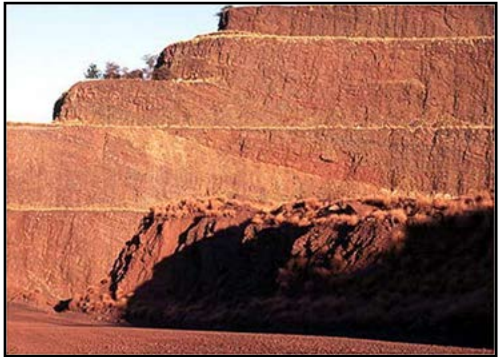
Figure 6: Benches in an open pit mine
