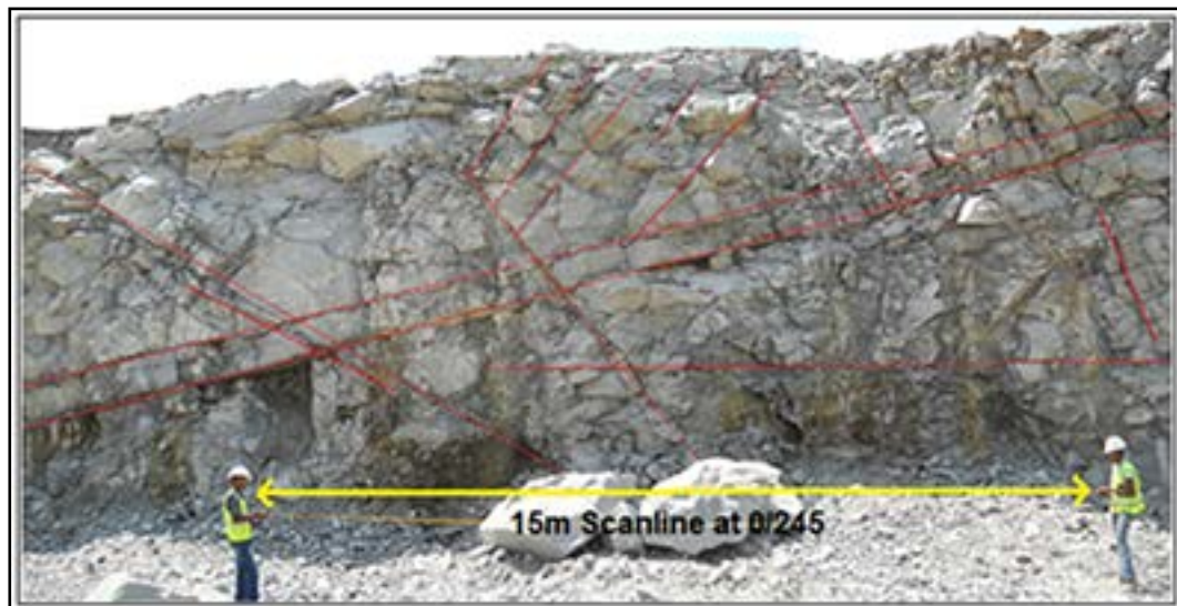
Figure 10: An example of a scanline.
