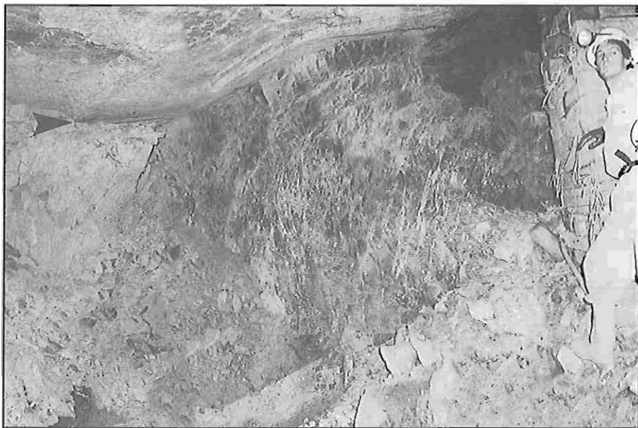
Figure 8.3.3 Photo-mosaic showing the face, viewed from position H (Figure 8.3.1) and looking updip. The timber packs on the right are situated to the east of the roll. The corresponding section is shown in Figure 8.3.2. The hangingwall fragmented during the rockburst. Most of the fallen rock was subsequently removed. Note the numerous fractures and joints in the face, and the smooth surface marking the parting above the collapsed brow.
