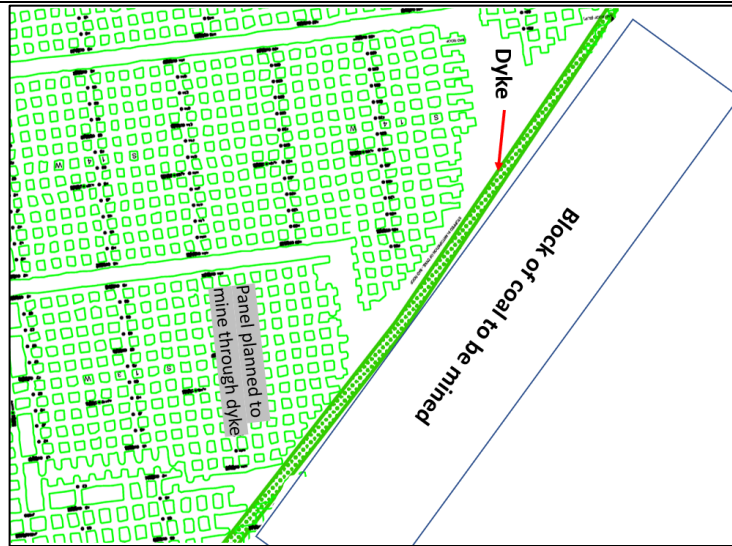
Figure 1-2: Plan showing mining against the dyke.
