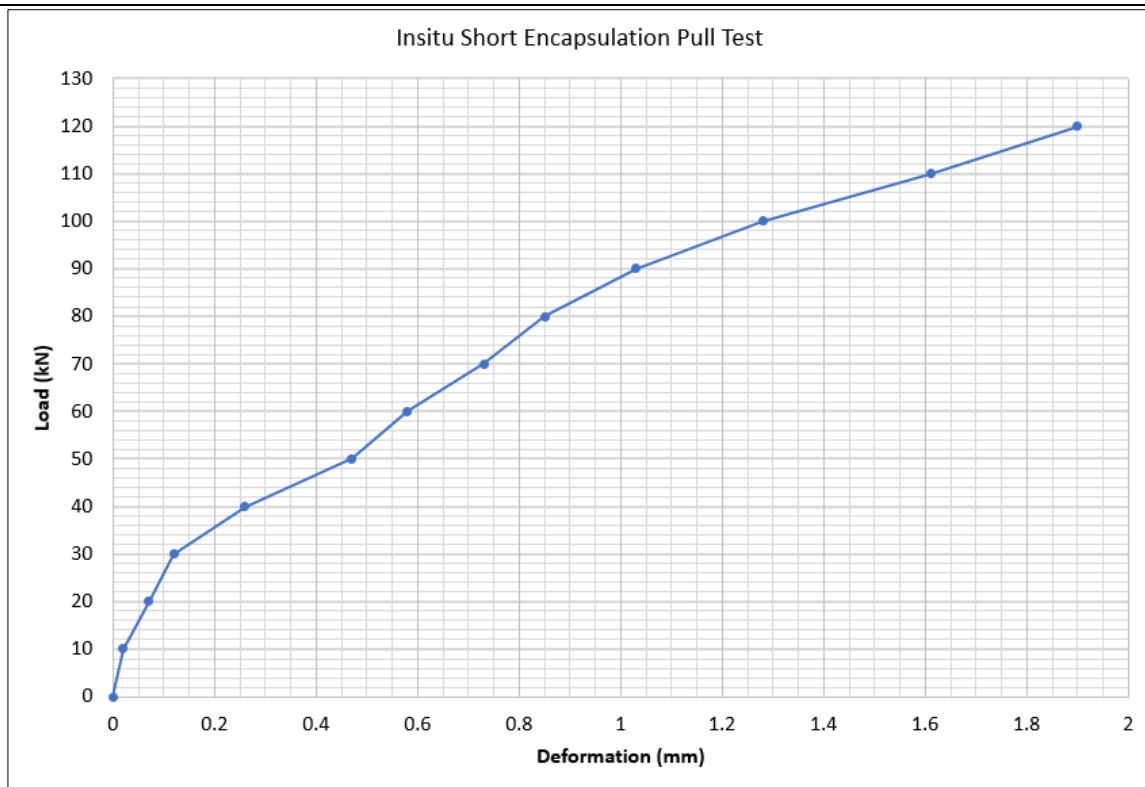
Figure 2-1: Insitu Short Encapsulation Pull Test Load-deformation curve.
