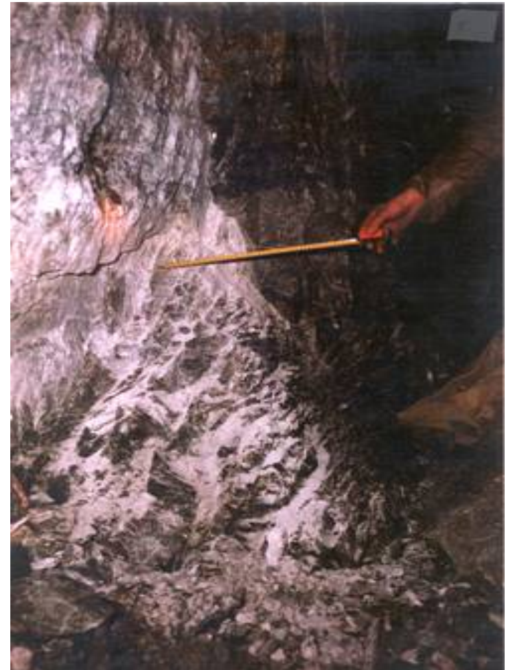
Figure 37: Ortlepp shears in the lava hangingwall (left) and through the VCR (right) at Mponeng – many years ago.
