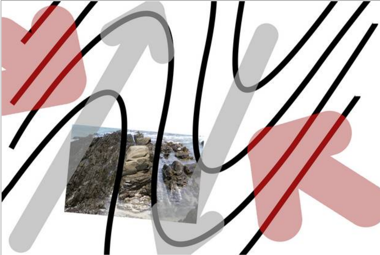
Figure 44: One possible interpretation of the origin of the extension fractures above. The red arrows depict tectonic load and the grey arrows depict material flow during folding.
