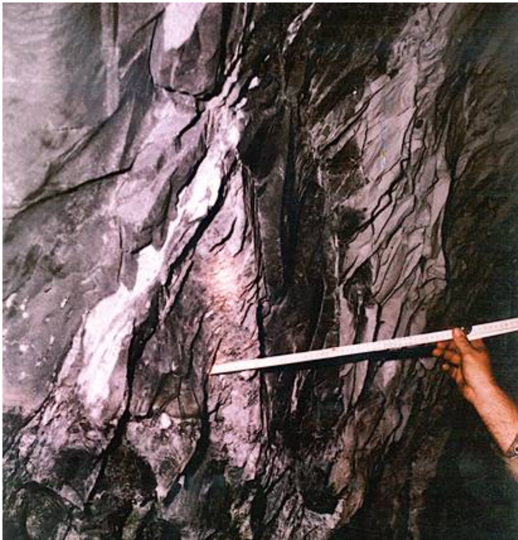
Figure 37: Ortlepp shears in the lava hangingwall (left) and through the VCR (right) at Mponeng – many years ago.
