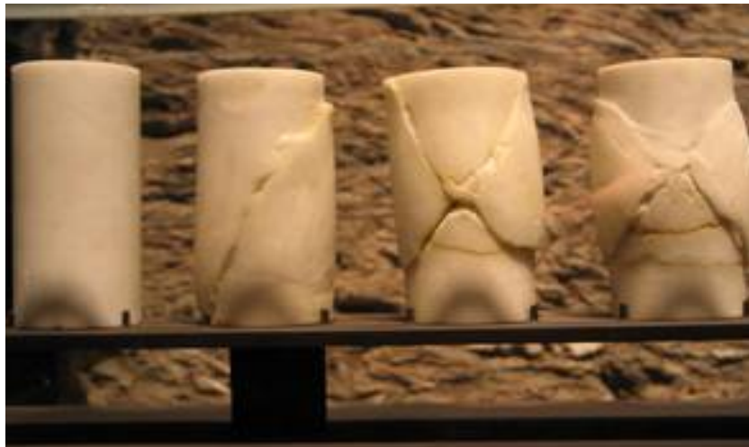
Figure 4: Self-explanatory pictures depicting pure shear vs simple shear, uni-axial vs triaxial deformation and high failure rate. Note that pure shear \neq simple shear
