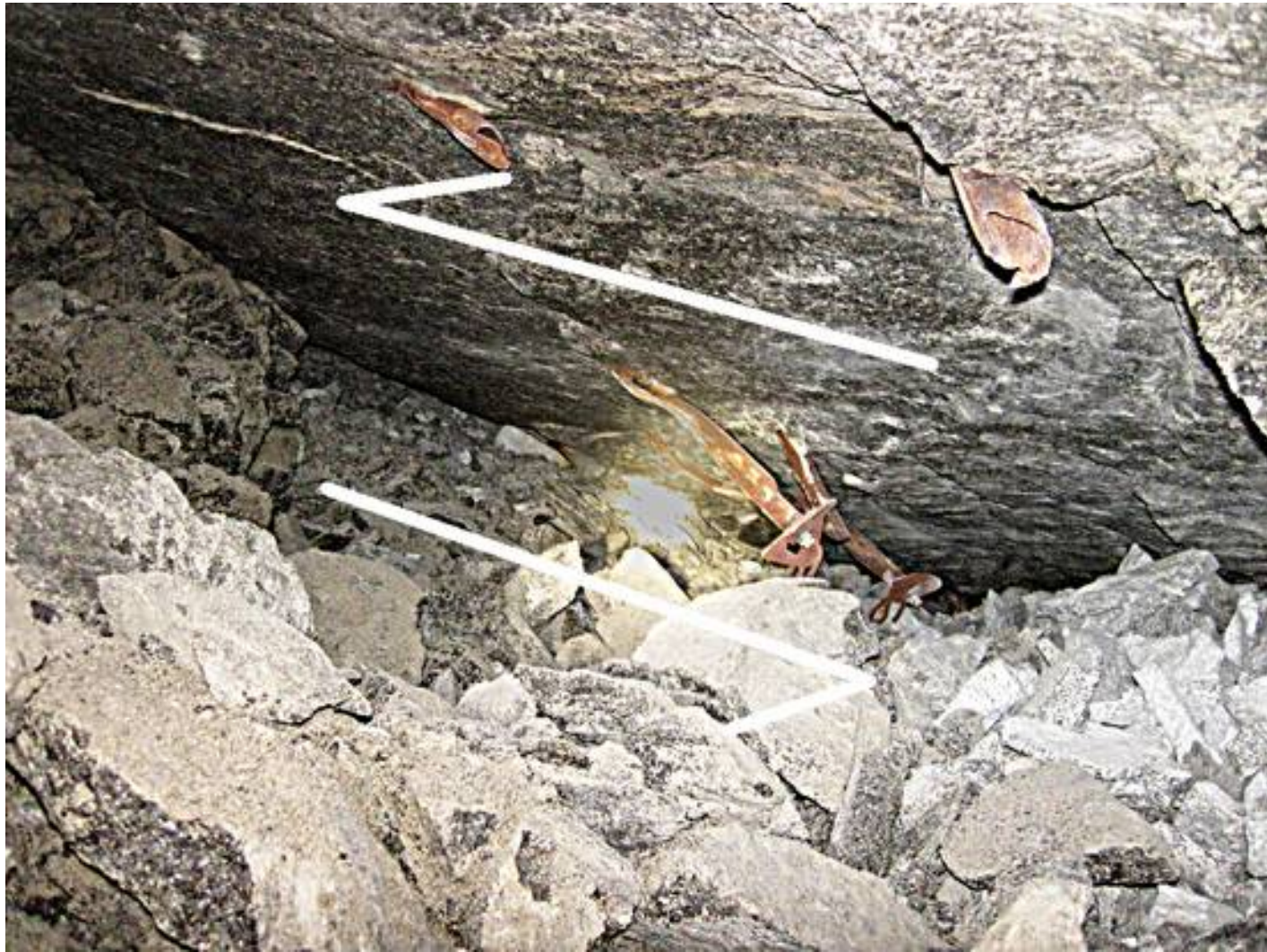
Figure 53: Rockburst mechanism at Siphu indicates principle stress is NS
