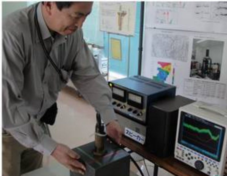
Figure 63: Hiroshi is compressing a cube of strong igneous rock in Prof. Ishi's laboratory and the measuring instrument is showing the elastic response. If Hiroshi could keep the same load for say 100 years, the elastic strain relax because the rock is not perfectly elastic.
