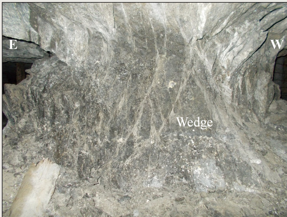
Figure 1: Photograph of a crush pillar from a trial site on Lonmin Platinum. Note the wedge-like structure visible where the fractures intersect. The fractures are concentrated predominantly towards the east, which was mined first.
