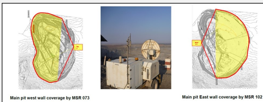
Figure 7: Radar monitoring of Main Pit.
