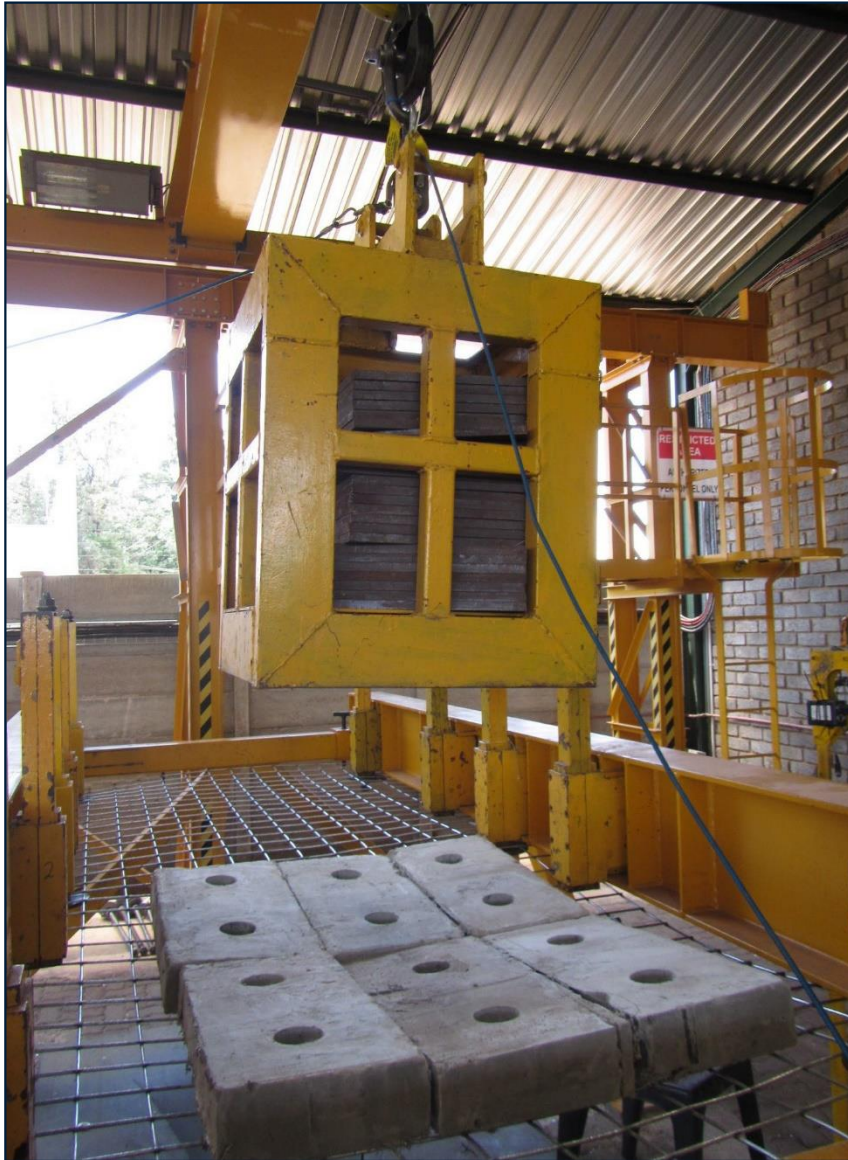
Figure 10. The dynamic test set up at the NCM drop test facility. A 1 tonne mass was dropped on the cellular lightweight concrete blocks to achieve a 4 kJ impact energy. The mesh was secured to the frame with bolts spaced 1.5 m apart in a square pattern
