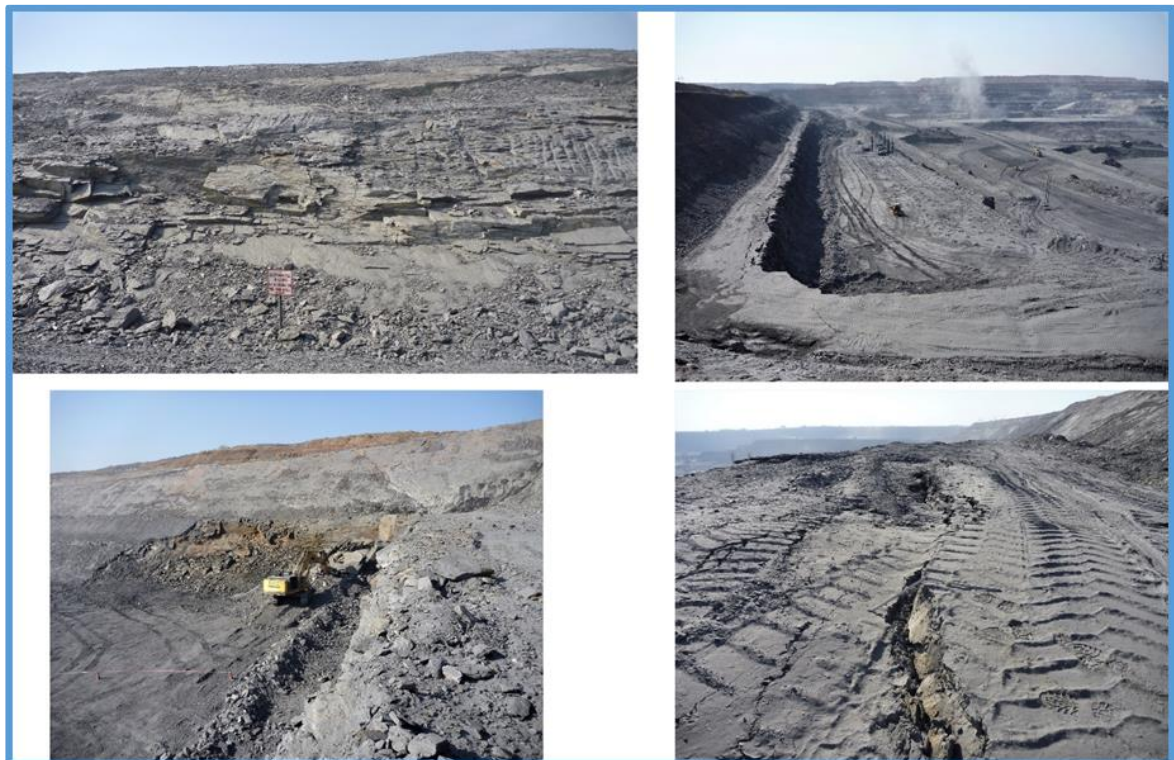
Figure 7: Typical failures in the South Wall
