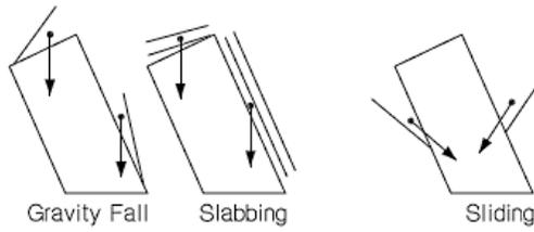
2) Next determine the gravity adjustment factor,  $C$ , based on the failure mode using the appropriate chart below.
